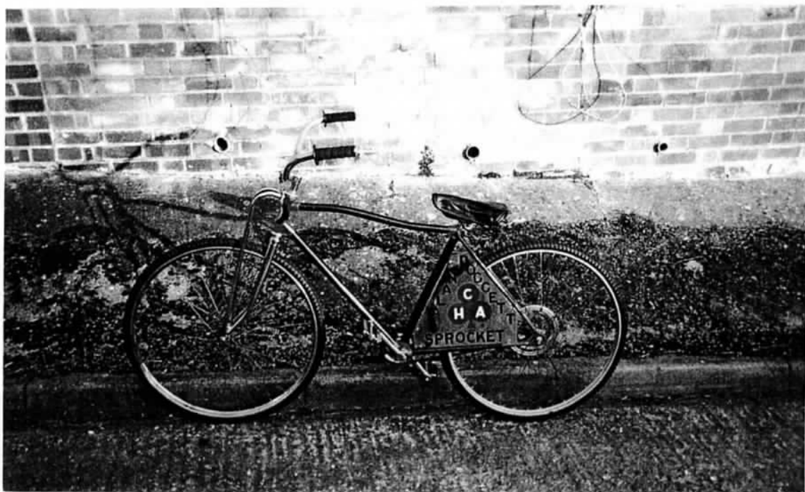
The 'Sprocket Special' Hand built in 1947 by Alan Doggett of Clay Hill Aces from second hand and salvaged parts. Featuring – Cut down frame, personalized \frac{1}{2} " gas pipe cow - horn handlebars, 'Skidway Gripster' Tyres, copper front fork stays, gearing 44 tooth crank x 22 tooth sprocket. Finished in Red/Black 'Robbialac' paint. No brakes, mudguards or projections
