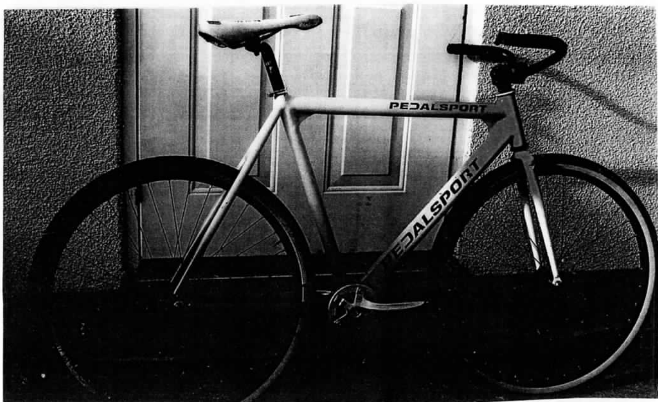
Ultra light weight special, hand built in Halifax for Mark Rushby of Pedal Sport. Featuring - frame made from Columbus Zonal Alloy with aero profile tubing, mountain - bike wheels, tyres, and chainset , 33 tooth chainwheel and 18 toothed sprocket fixed on a cassette splined hub.
